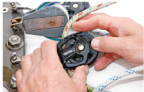
A good quality, open-sheave turning block with ball bearings makes a world of difference when handling lines.
